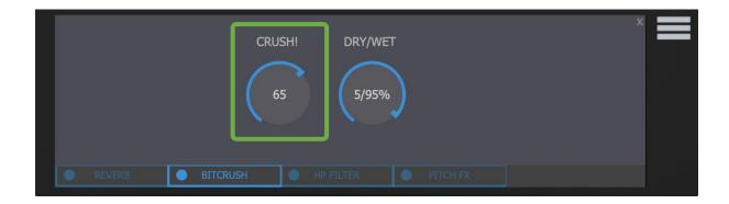
It reduces the sample rate, from your selected sample rate in your DAW to 2000Hz. The parameter knob at 0 % changes nothing, at 100% you get the maximum sample rate reduction.
