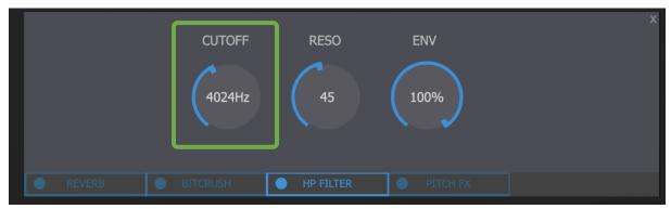
Determines the cutoff frequency of the HP Filter Use this fader to set the cutoff frequency.
