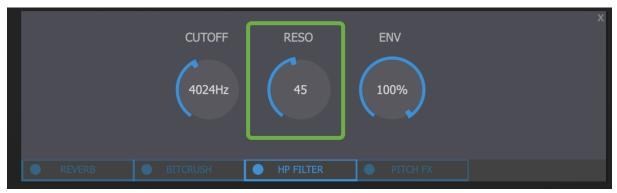
In a hi pass filter, resonance emphasizes signals at the cutoff frequency.
