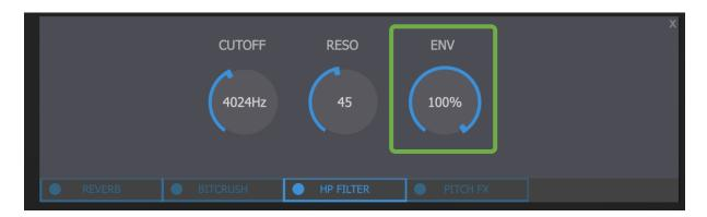
In the filter section that sets the amount of envelope applied to the cutoff frequency. Use this fader to set the amount of envelope applied to the cutoff frequency of the filter. Filter envelope is controlled by the audio input amplitude signal.
