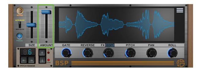
The "Slice Amount" defines the balance between re-arranged slices and direct signal from the input.
