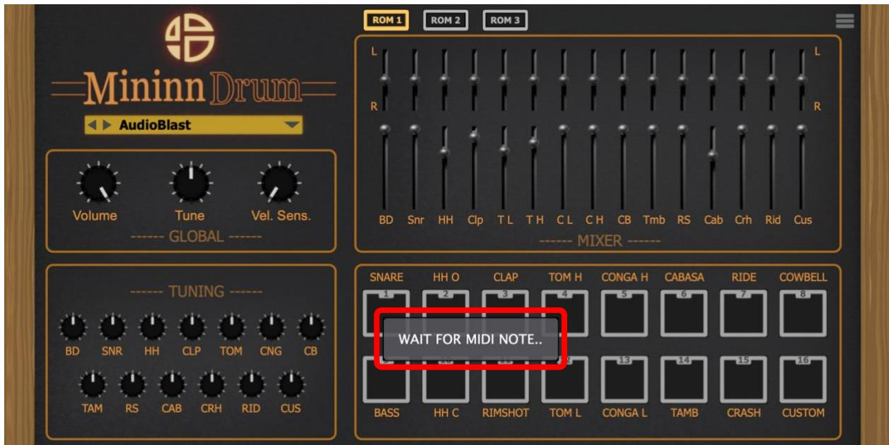
When WAIT FOR MIDI NOTE appears just push the selected note on your controller and the pad will be automatically assigned to it.
